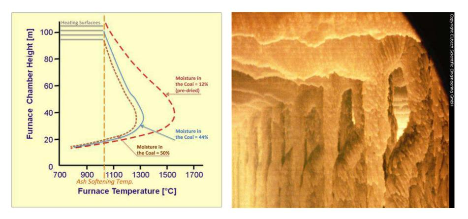
→ The Furnace Exit Gas Temperature (FEGT) must be kept bellow the Ash Softening Temperature
