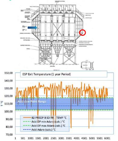
→ Due to combustion of particular imported coals the flue gas temp. is critically close to the acid dew point and in some periods bellow it
